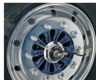
TIRE PRESSURE MONITORING AND INFLATION SYSTEMS ensure the ideal tire pressure and prevent unnecessary additional consumption.
