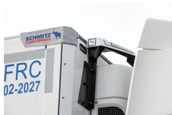
THE FRONT WING SYSTEM makes the roof area between the traction unit and the trailer less susceptible to turbulence.
