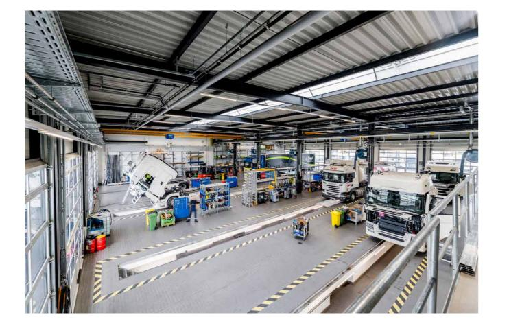
KNIRSCH'S SCHUTTERWALD BRANCH is equipped with a total of seven service bays, including three with maintenance pits. All seven can be double-stacked.
