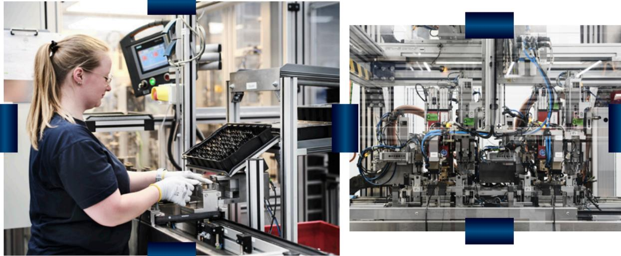
The coil body blister packs are brought to the second workstation manually. Once there, a production worker removes the individual components from the pack and places them in a workpiece holder. The worker also attaches cables for assembly in the machine which the holder then enters automatically. The machine strips
