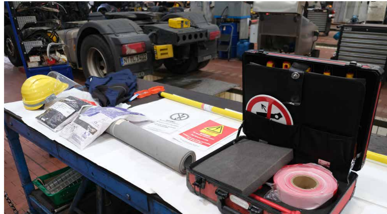
HARD HATS WITH VISORS , insulating mats and special gloves are among the other required PPE items.
