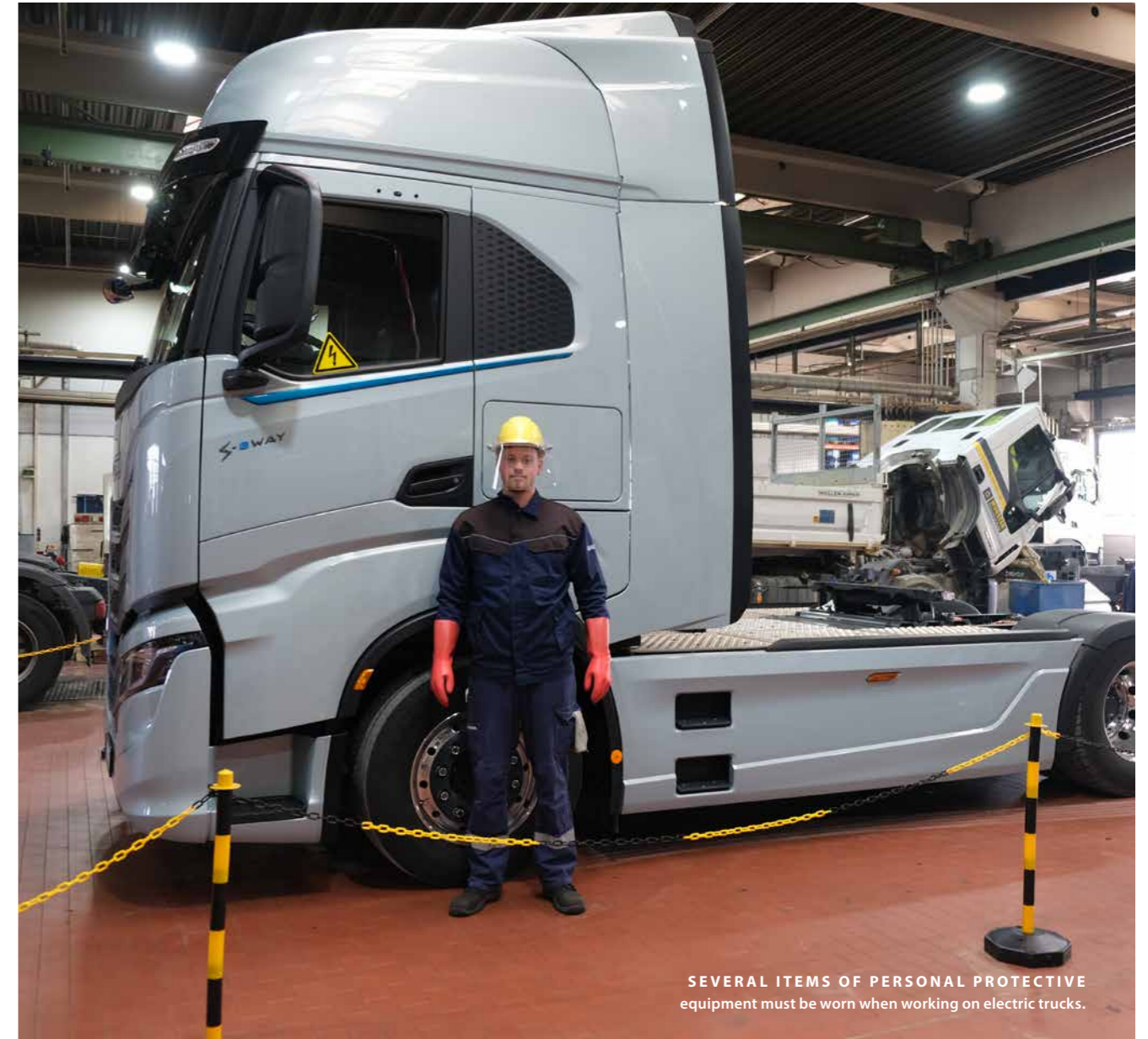
THE PERSONAL PROTECTIVE EQUIPMENT includes antistatic and flame-retardant workwear.
