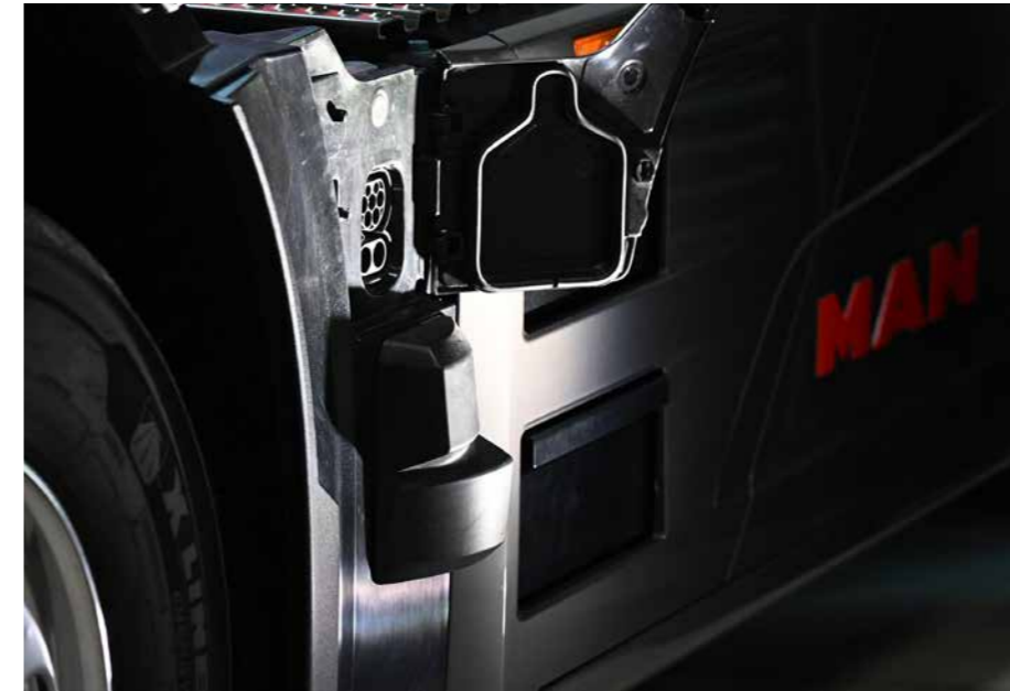
CCS (LEFT) AND MCS SOCKETS (BELOW) COMPARED In the future, MCS will enable charging at up to 3.75 megawatts, while CCS is restricted to less than 500 kW.
