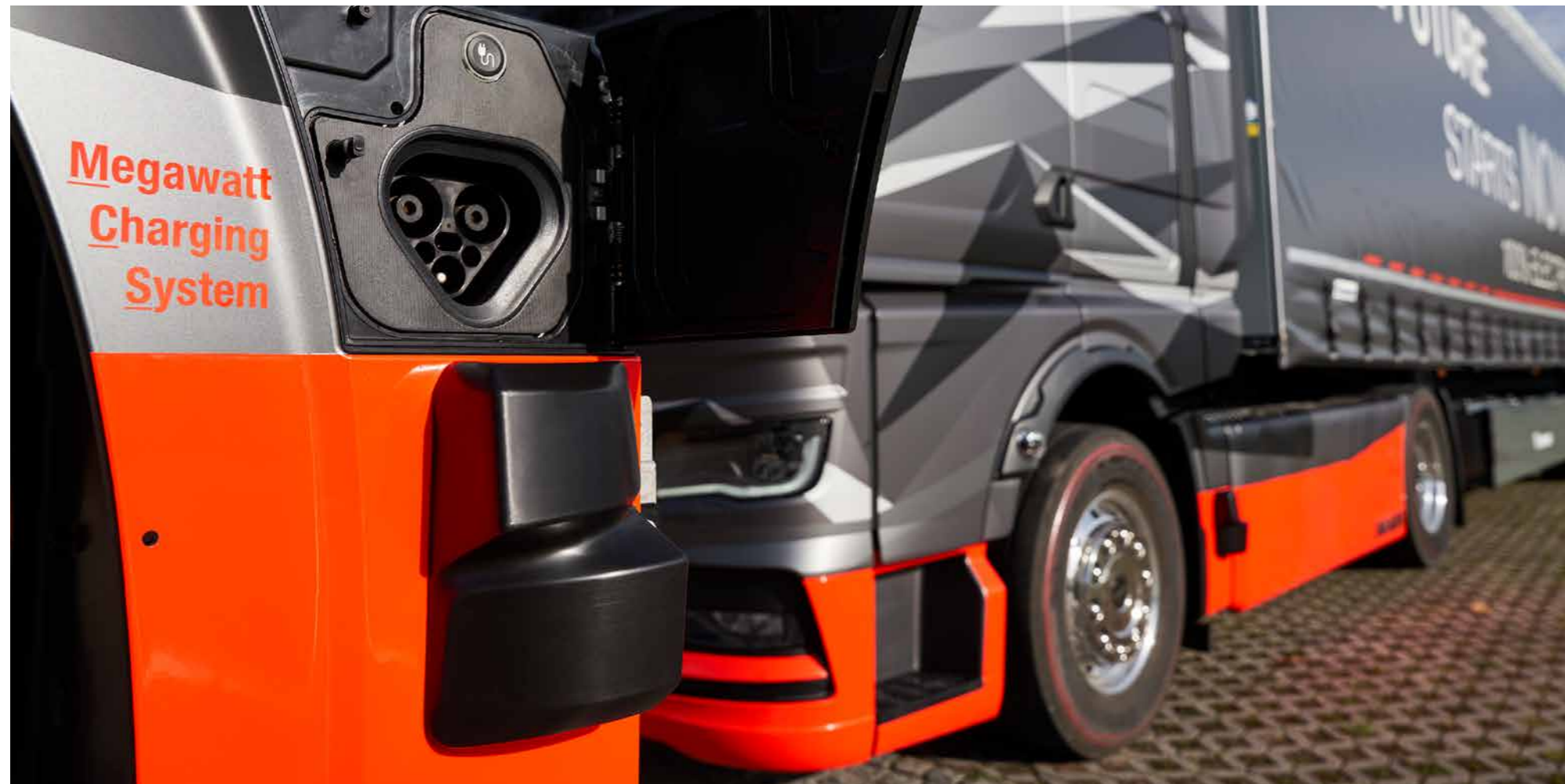
CCS (LEFT) AND MCS SOCKETS (BELOW) COMPARED In the future, MCS will enable charging at up to 3.75 megawatts, while CCS is restricted to less than 500 kW.
