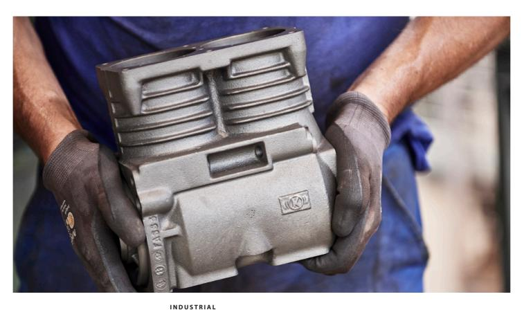
REMANUFACTURING involves complex cleaning processes and replacement of worn components.
